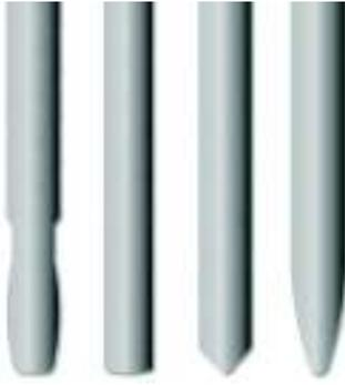
Here are drawings of the profiles of four circle-segment tool types. Seen here from left to right are barrel, lens, taper and oval forms.
