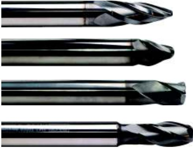
Photos of the different circle-segment tool types. The lens tool (third from top) has its large-radius cutting edge along the tool tip.
