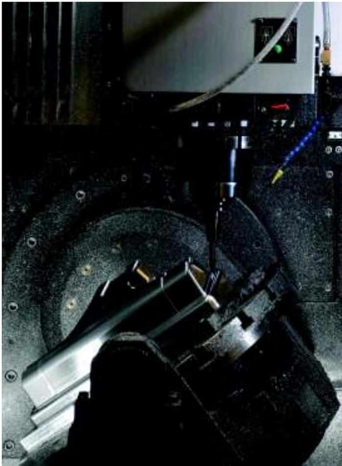
Circle-segment tools all but need five-axis machines, particularly in machining of die and mold forms, to keep them cutting at the angles they require. These tools realize the promise made possible through sophisticated machine motion plus sophisticated programming.
