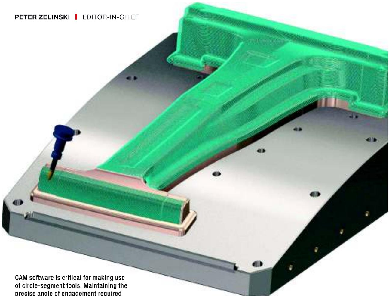
CAM software is critical for making use of circle-segment tools. Maintaining the precise angle of engagement required demands tool paths tailored to each of the different circle-segment tool types.
